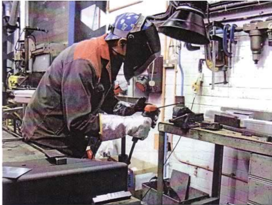
(c) Operator making a vertical weld
