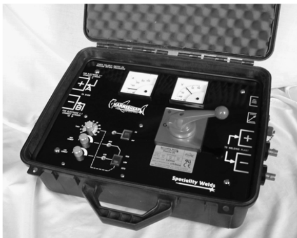
Fig 1: The control panel with isolation switch, amp/volt meters and the Hammerhead control device (bottom left)
