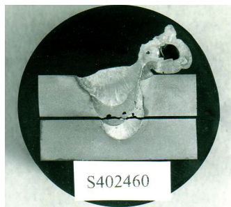
Image shows a spot weld and 'flash' test piece cut through the centre and macro polished.
