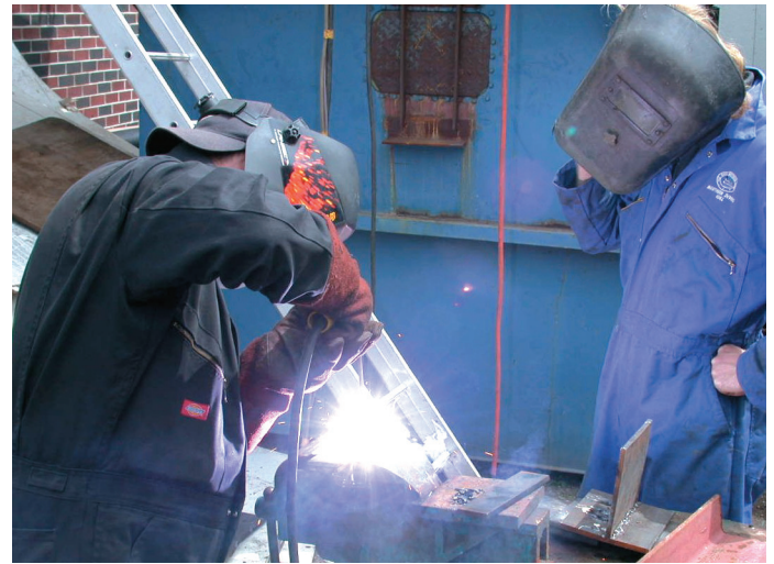
The Hammerhead system has the added advantage of also working well for welding above water.
